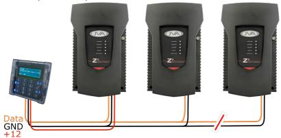
By disconnecting each Z-Series Energizer in turn from the keypad bus (shown in the above diagaram) you can check to see how each Z-Series device behaves under comms fail conditions. This way, you can test to see that the relays have been configured correctly for comms fail. Once you are satisfied that each Z-Series device is configured correctly you can begin to wire them to the real fence.
